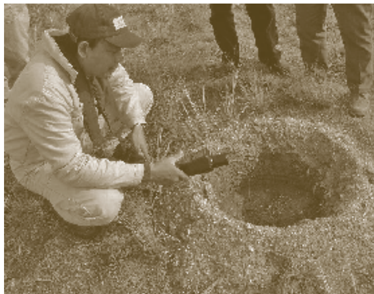
FIELD USE OF HAND-HELD TOOL FOR RADIONUCLIDE SURVEY AND IDENTIFICATION
