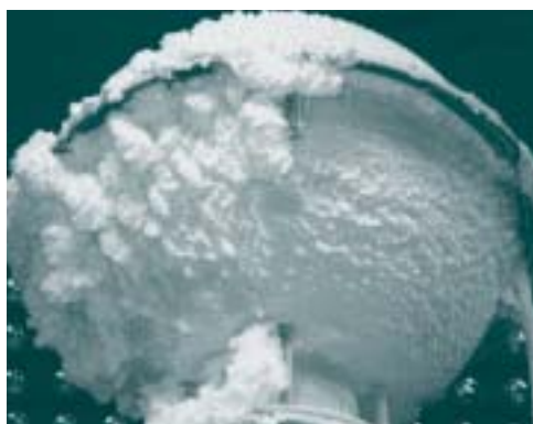
FIGURE 1: ICE RIMING DURING THE WIND TUNNEL TESTS IN VIENNA (AUSTRIA)
